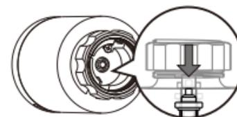
3 Install TRV with M30\*1.5 screw thread Interface of valve .Tighten the plastic ring.
